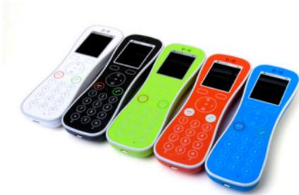
The KIRK Butterfly Handset Series is a basic wireless handset designed for office environments with the most important features and functionalities of basic wireless telephony and messaging.
